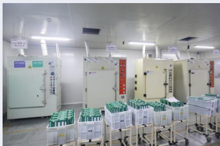
Finished product moisture removal and leveling equipment
