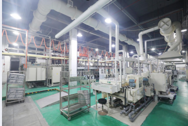
Auto outer layer de-filming and etching de-tinning line
